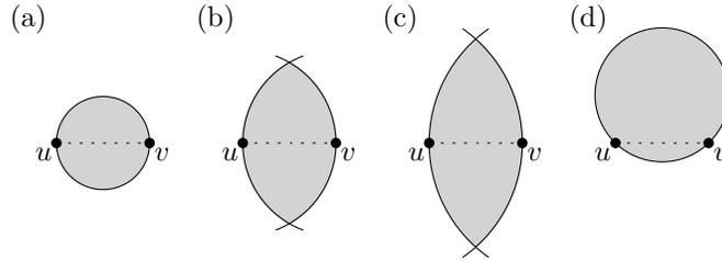
Figure 1: Two points  $u$  and  $v$ . Indicated by shading: (a) their Gabriel disk (which coincides with their  $\beta$ -region for  $\beta = 1$ ), (b) their  $\beta$ -region for  $\beta = 2$ , (c) their  $\beta$ -region for  $\beta = 3$ , and (d) one of their Delaunay disks.
