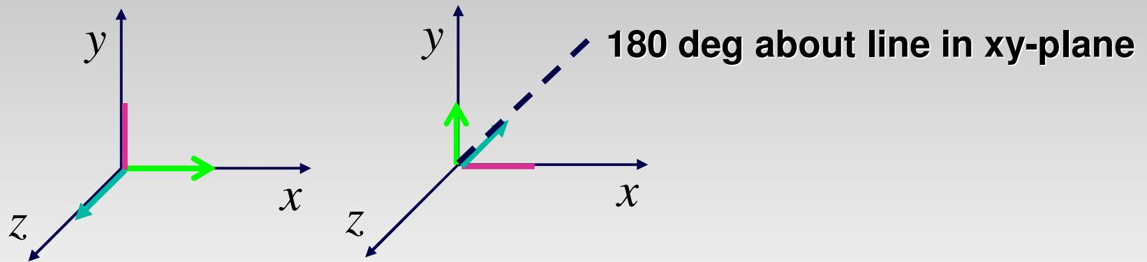
$$Rot(\vec{k}, \theta) = \begin{bmatrix} k_x^2 v + c & k_x k_y v - k_z s & k_x k_z v + k_y s \\ k_x k_y v + k_z s & k_y^2 v + c & k_y k_z v - k_x s \\ k_x k_z v - k_y s & k_y k_z v + k_x s & k_z^2 v + c \end{bmatrix}$$
