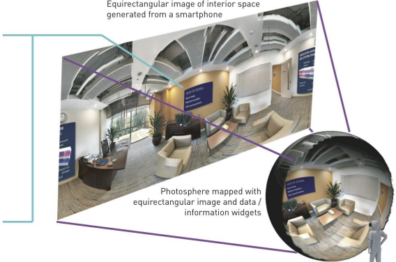
One can interact with data and widgets via a VR headset and smartphone (i.e., Google Cardboard) or on in a generic 2D web browser (i.e., Google StreetView-type interaction)
