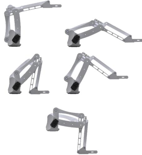
Fig. 6. Motion capabilities of the basic palletizing robot design under consideration. Images are of my robot arm design *EvoArm*, rendered using CAD software.
