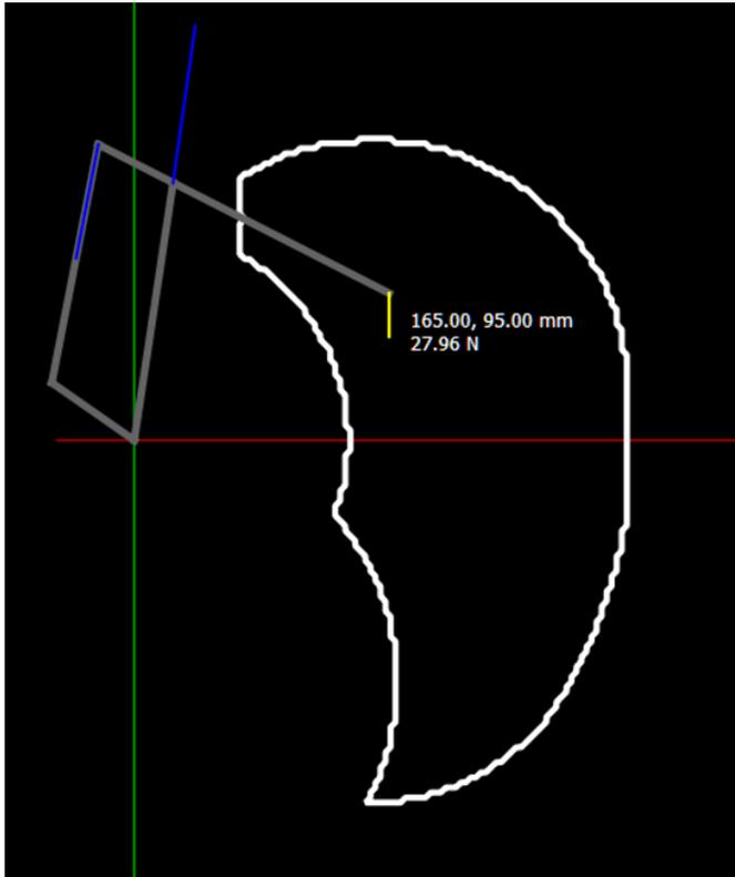
Fig. 7. Simple outline view of a workspace, with a visualization of the robot arm itself also overlaid (this appears while hovering the mouse over the workspace)
