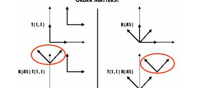
$$Ta Tb = Tb Ta, \text{ but } Ra Rb \neq Rb Ra \text{ and } Ta Rb \neq Rb Ta$$
