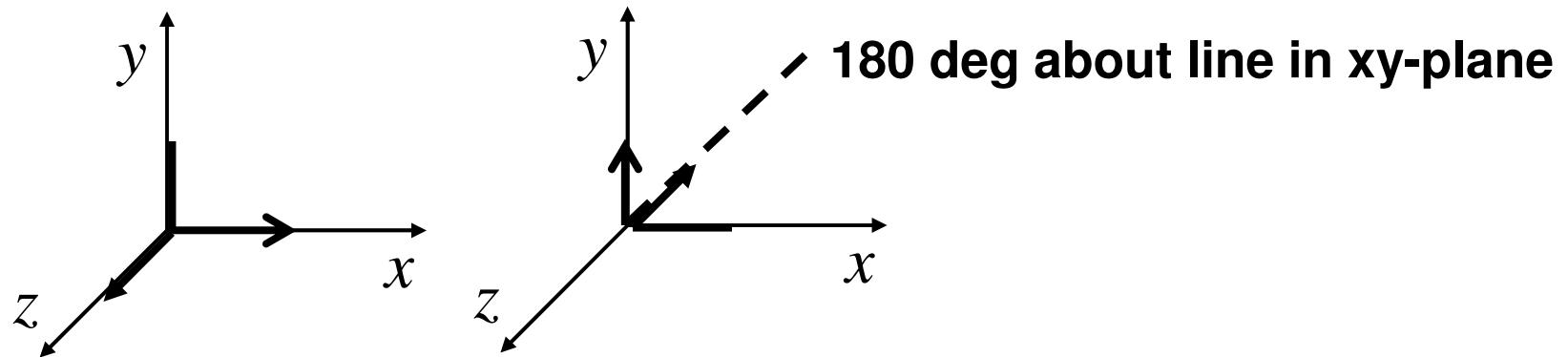
$$Rot(\vec{k}, \theta) = \begin{bmatrix} k_x^2 v + c & k_x k_y v - k_z s & k_x k_z v + k_y s \\ k_x k_y v + k_z s & k_y^2 v + c & k_y k_z v - k_x s \\ k_x k_z v - k_y s & k_y k_z v + k_x s & k_z^2 v + c \end{bmatrix}$$
