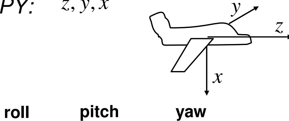
$$R_{RPY} = \text{Rot}(z, \alpha) \text{Rot}(y, \beta) \text{Rot}(x, \gamma)$$
