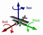
Yaw is rotating horizontally with respect to your current position, like steering a car or shaking your head for no. Pitch is rotating vertically with respect to your current position, like nodding your head up and down for yes. Roll is tipping left or right by rotating around your current front-to-back axis, like tilting your head so your ear touches your shoulder. See also the animated illustration at http://www.nasm.si.edu/galleries/gal109/NEWHTF/PITCH.HTM
