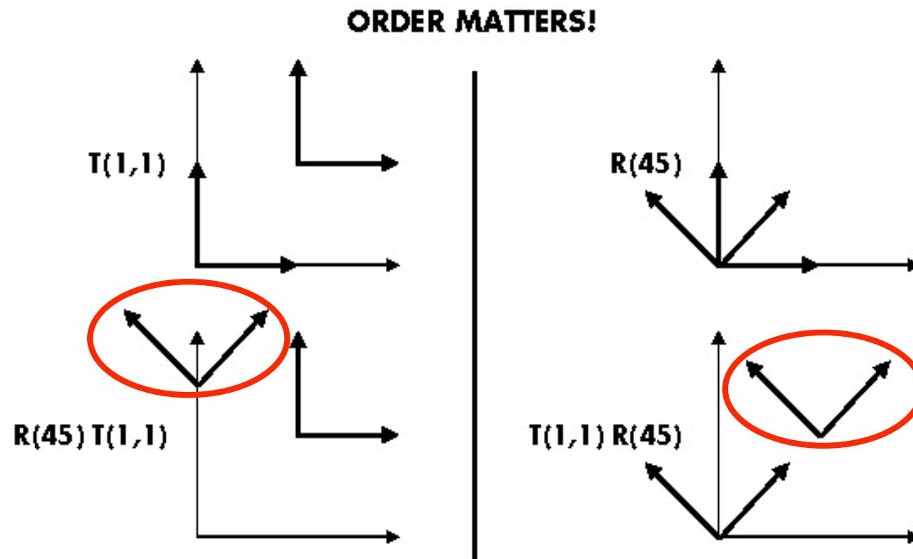
$T_a T_b = T_b T_a$ , but  $R_a R_b \neq R_b R_a$  and  $T_a R_b \neq R_b T_a$
