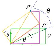
$$\begin{aligned} x' &= x \cos \theta - y \sin \theta \\ y' &= x \sin \theta + y \cos \theta \\ z' &= z \end{aligned}$$
