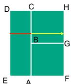
first portion of the scanline is interpolated between DE and AC
