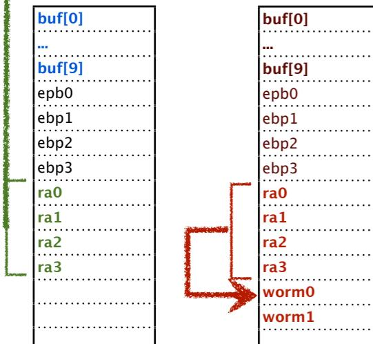
\* The worm is loaded onto stack
