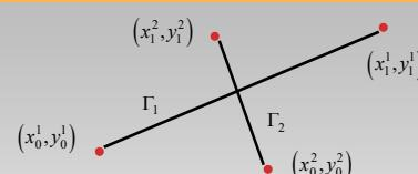
$$G_1 = \begin{cases} x^1(t) = x_0^1 + (x_1^1 - x_0^1)t \\ y^1(t) = y_0^1 + (y_1^1 - y_0^1)t \end{cases} \quad t \in [0,1] \quad G_2 = \begin{cases} x^2(r) = x_0^2 + (x_1^2 - x_0^2)r \\ y^2(r) = y_0^2 + (y_1^2 - y_0^2)r \end{cases} \quad r \in [0,1]$$
