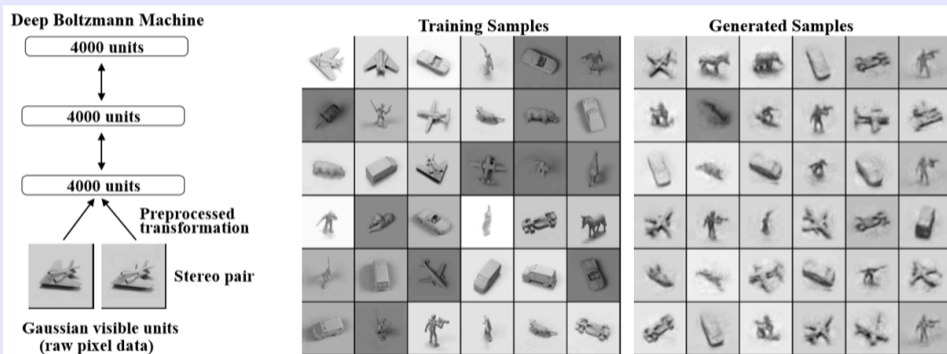
Figure 5: Left: The architecture of deep Boltzmann machine used for NORB. Right: Random samples from the training set, and samples generated from the deep Boltzmann machines by running the Gibbs sampler for 10,000 steps.
