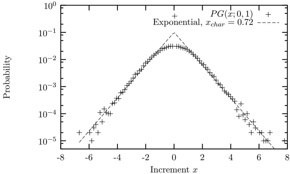
Figure B.4: Discrete Brownian motion with Poisson-distributed jump intervals has tails which fall off exponentially (with a decay constant of 0.72), instead of as  $e^{-x^2}$ , when sampled at regular intervals ( $\Delta = 1$ ).
