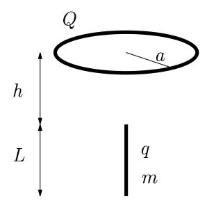
In a laboratory, a ring of charge  $Q=8\,\mu\mathrm{C}$  with radius  $a=30\,\mathrm{cm}$  levitates a charged rod of length  $L=20\,\mathrm{cm}$  and mass  $m=100\,\mathrm{g}$ , as shown above. The top of the floating rod is  $h=10\,\mathrm{cm}$  below the center of the ring. (a) Draw a free body diagram for the rod in equilibrium. (b) Assuming it is uniformly distributed, what is the total charge q of the rod?
