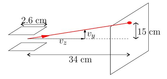
From the diagram we see that the speed and displacement triangles are similar so, after deflection,
