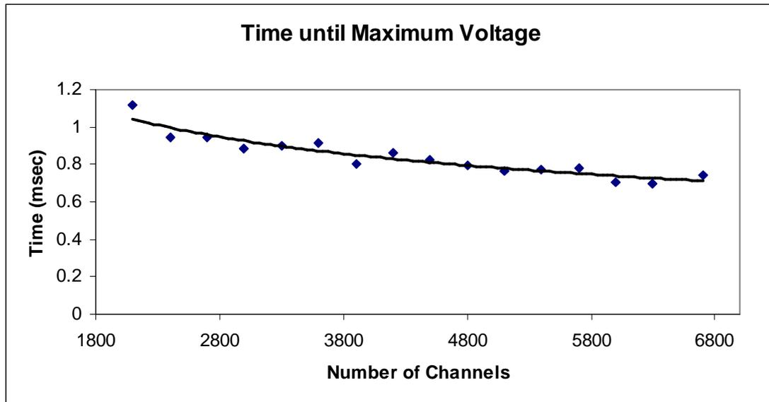
Figure 5. A graph showing the time until maximum voltage attained during our simulation of the action potential plotted against the number of sodium and potassium channels in the membrane. The model was run starting from rest at -65mV and then given a depolarizing pulse to -45mV.
