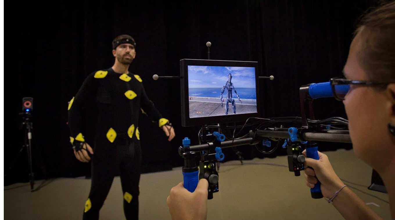
Virtual camera registered in the real world (using marker-based motion capture)
