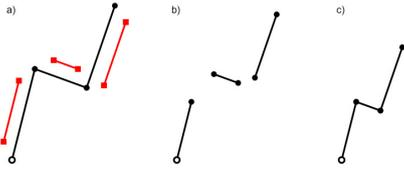
**Figure 1:** a) Mass spring system with 1 constrained point (white point). Red lines show the maximum allowable lengths of each spring. At this point an initial guess of forces is calculated b) The impulse forces from step 1 are applied to each spring individually. Shared nodes disagree on their final positions since they are being pulled in different directions. c) Step 3 stitches the system back together, respecting the constrained points and lengths of springs.
