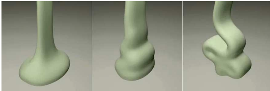
Figure 3.3: Three different simulations of a long sheet of fluid falling under gravity demonstrating the influence of viscosity on buckling; from left to right viscosity values are 0.2, 1, and 5.
