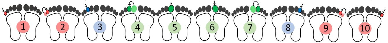
Fig. 2: Final design of HapToes for both feet. For numbers 1, 3, 5, 6, 8 and 10, a long vibration of 1200 ms is rendered on the targeted toe (darker color). For the remaining numbers 2, 4, 7 and 9, a short vibration of 400 ms is rendered on the closest edge toe, followed by a longer vibration of 800 ms on the targeted toes (darker color).
