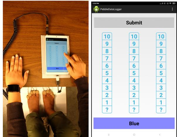
Fig. 3: Experiment setup and tablet UI for entering responses. In the experiment, the feet are obscured by the table, included here for illustration purposes.
