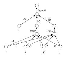
The function can be represented as  $(x \wedge y) \vee (\neg x \wedge z)$
