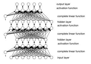
• Each hidden unit outputs a linear function of its inputs followed by a non-linear activation function.
