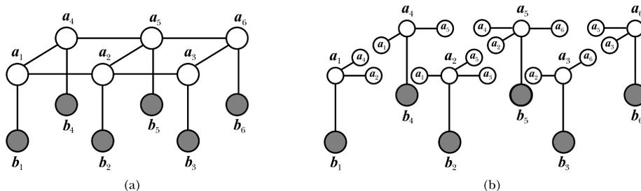
**Fig. 2.** (a) A sample Markov random field with 6 blob sites. We have omitted the  $n$  subscript. The  $\Phi$  potentials are defined on the vertical lines, and  $\Psi$  on the horizontal lines. (b) The corresponding pseudo-likelihood approximation.
