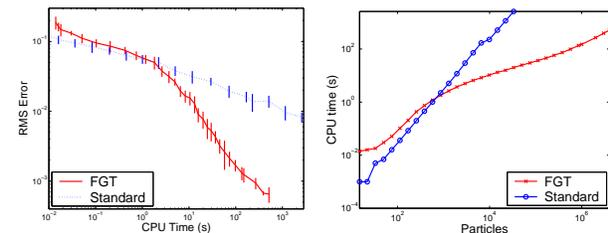
Figure 6: Particle-smoothing results on synthetic data, shown on a log-log scale for clarity. The data in both plots stem from the same experiment. For the same computation cost, FGT achieves an RMSE two orders of magnitude lower. We are able to smooth with as many as 4,000,000 particles with this method!
