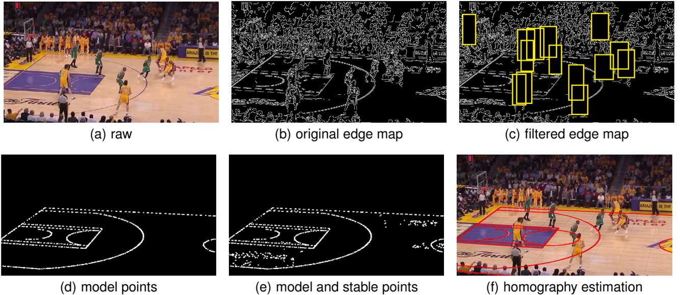
Fig. 6. Estimating the homography in basketball videos. (a) A raw video frame. (b) Canny edges [48] of the frame. (c) Filtered Canny edges by dropping edges caused by players. (d) The original model points. (e) The original model point set augmented by stable points. (f) Homography estimation results by a variant of Iterated Closest Point (ICP) [49].
