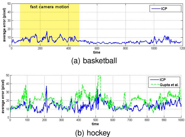
Fig. 11. Homography estimation results in (a) basketball, and (b) hockey, compared to [47]. Errors are measured by the average distance between points transformed by the annotated and estimated homography.
