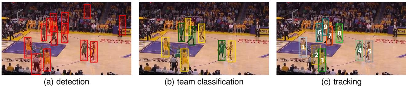
Fig. 1. (a) Automatic player detection generated by the DPM detector [29]. (b) Automatic team classification. Celtics are in green, and Lakers are in yellow. (c) Automatic tracking by associating detections into tracklets. Numbers represent the track ID not player identities.
