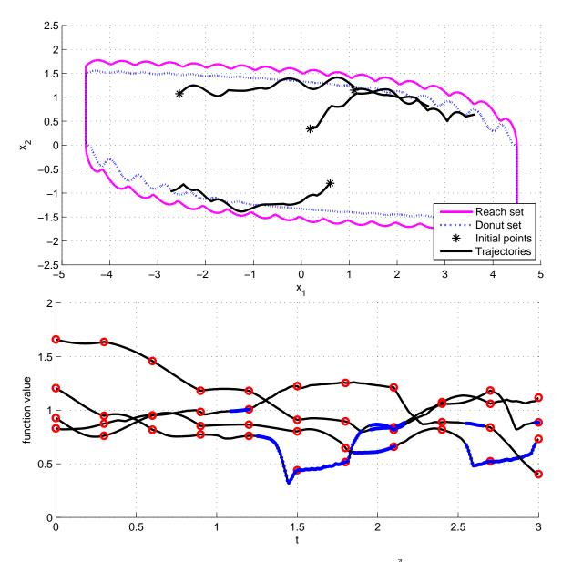
Figure 8: Sample trajectories using the aggressive safe policy  $\mathcal{U}_{ctrl}^{\nearrow}$  for  $\delta = 0.3$ . Top: Trajectories  $x(\cdot)$  in phase space overlaid on the state space partition. Bottom row:  $\psi_{\mathcal{S}_{\infty}}(x(t))$  versus t. Sample times are shown as red circles, and periods during which  $x(t) \in \mathcal{S}_{ctrl}$  are shown with blue dots.
