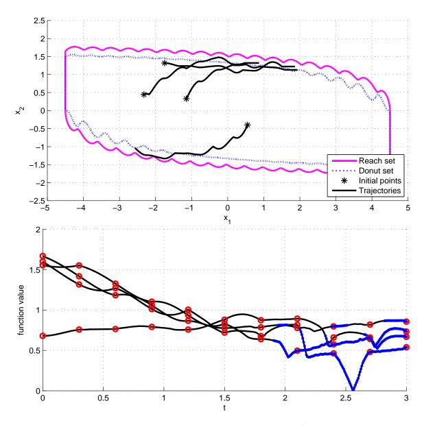
Figure 7: Sample trajectories using the permissive safe policy  $\mathcal{U}_{ctrl}^{\rightarrow}$  for  $\delta = 0.3$ . Top: Trajectories  $x(\cdot)$  in phase space overlaid on the state space partition. Bottom row:  $\psi_{\mathcal{S}_{\infty}}(x(t))$  versus t. Sample times are shown as red circles, and periods during which  $x(t) \in \mathcal{S}_{ctrl}$  are shown with blue dots.
