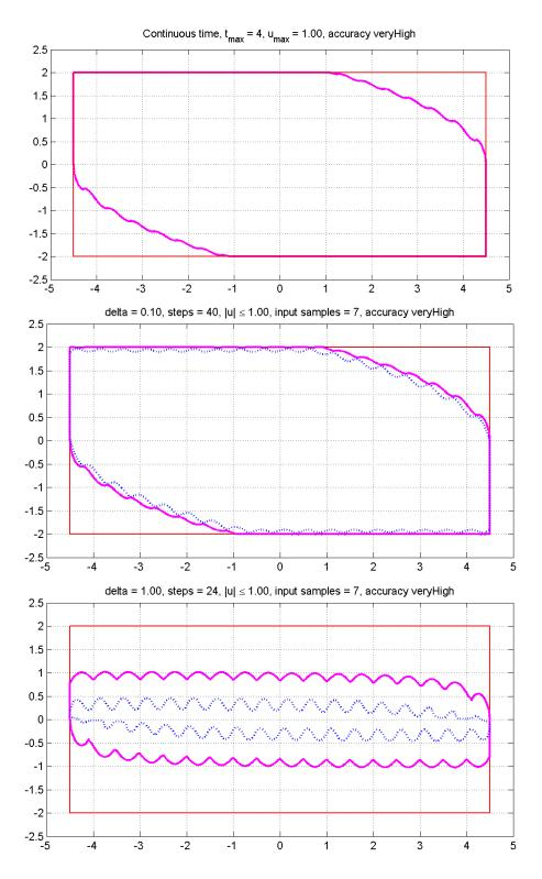
Figure 6: The effect of  $\delta$  on the spatial partition. Top: Traditional reachability with continuous state feedback and measurable control signals (T = 4). Middle: Sampled data with  $\delta = 0.1$ , N = 40 (T = 4). Bottom: Sampled data with  $\delta = 1.0$ , N = 24 (T = 24).
