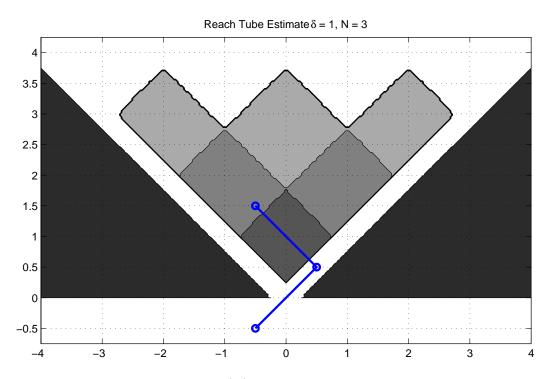
Figure 2: A demonstration that  $\mathcal{R}_N^-(\mathcal{T})$  may include states which can avoid hitting the terminal set. The terminal set  $\mathcal{T}$  is the two black triangles. The remaining shaded regions are  $\mathcal{R}_k^-(\mathcal{T})$  for k = 1, 2, 3 (darkest to lightest). The blue line shows a trajectory starting from within  $\mathcal{R}_2^-(\mathcal{T})$  which nonetheless avoids the terminal set. The input is sampled at the points marked by small circles.
