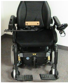
Figure 1. NOAH wheelchair system (commercially available wheelchair equipped with stereo-vision camera and laptop)
