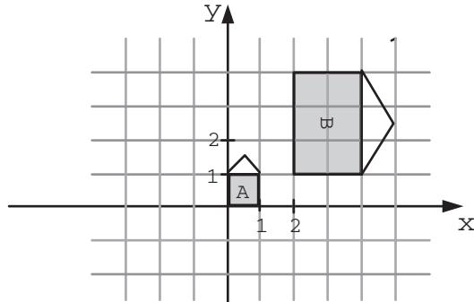
3. [6 marks] Given 2 points  $\mathbf{a} = (a_x, a_y)$  and  $\mathbf{b} = (b_x, b_y)$ , where  $b_y > a_y$  like those in the figure below, give pseudocode to rasterize the edge (as done in triangle rasterization). That is, for each scanline between  $y = a_y$  and  $y = b_y$ , compute the pixel at which the line segment intersects the scanline.
