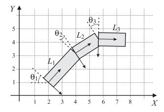
(a) (4 marks) Given a point (a, b) on the finger tip, in the local coordinate frame of part  $L_3$ , write the sequence of transformation matrices that will transform this point to the world coordinate frame of reference.
