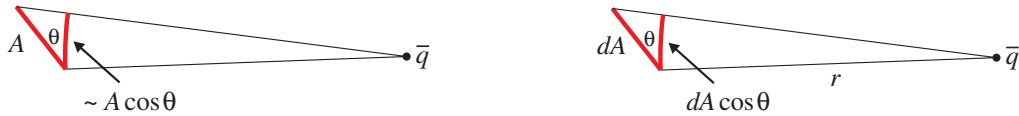
Figure 4: Foreshortening in 2D. Left: For a patch with area A , seen from a point \bar{q} , the patch’s foreshortened area is approximately A \cos \theta . This is an approximation, since the distance r varies over the patch. The angle \theta is the angle between the patch normal and the direction to \bar{q} . Right: For an infinitesimal patch with area dA , the foreshortened area is exactly dA \cos \theta .
