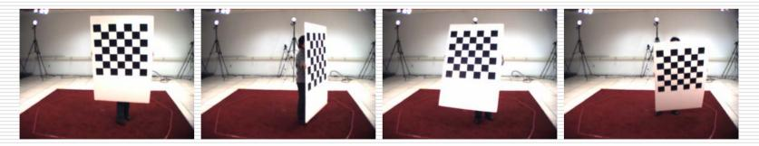
Extrinsic calibration of video cameras (R<sub>c</sub>, T<sub>c</sub>)
