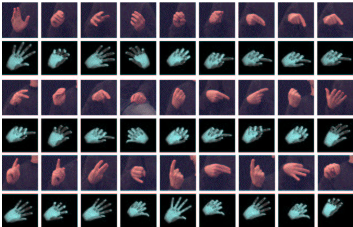
Figure 5: Reconstruction obtained from performing hand segmentation in a human subject. The two top pairs of rows show good reconstruction while the bottom pair show examples of bad performance. Reconstruction is shown from a fixed viewpoint (latitude 0-longitude \pi rads.).
