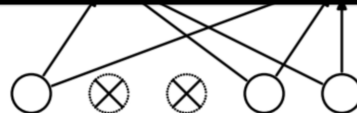
After Applying Dropout
