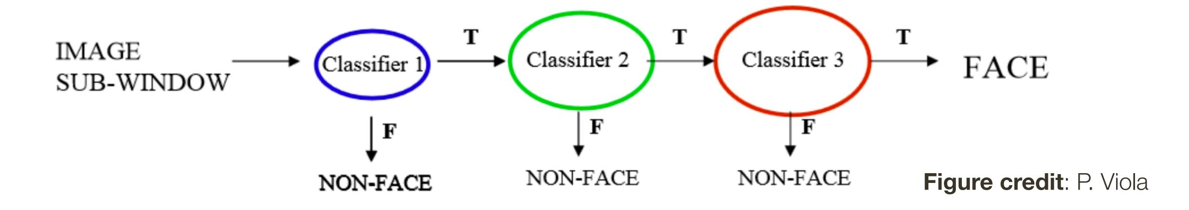
To make detection **faster**, features can be reordered by increasing complexity of evaluation and the thresholds adjusted so that the early (simpler) tests have few or no false negatives
