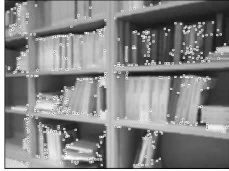
Figure 1: A corner detection sample result.
