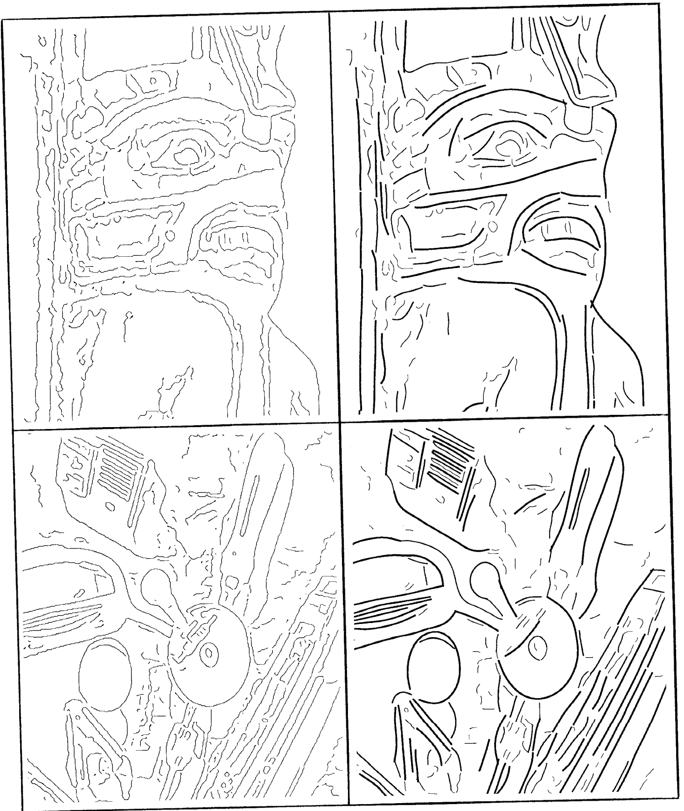
Figure 6: On the left are edges detected by the Canny edge finder. On the right are the final curve segments output by the multi-scale smoothing and segmentation algorithm. The thickness of each curve is proportional to the scale of smoothing selected for that curve.
