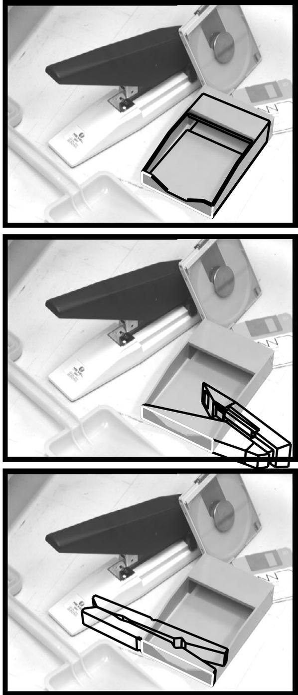
Figure 1: A single image grouping (white lines) indicates several possible model matches (black lines) via indexing. At most one of these may be valid.
