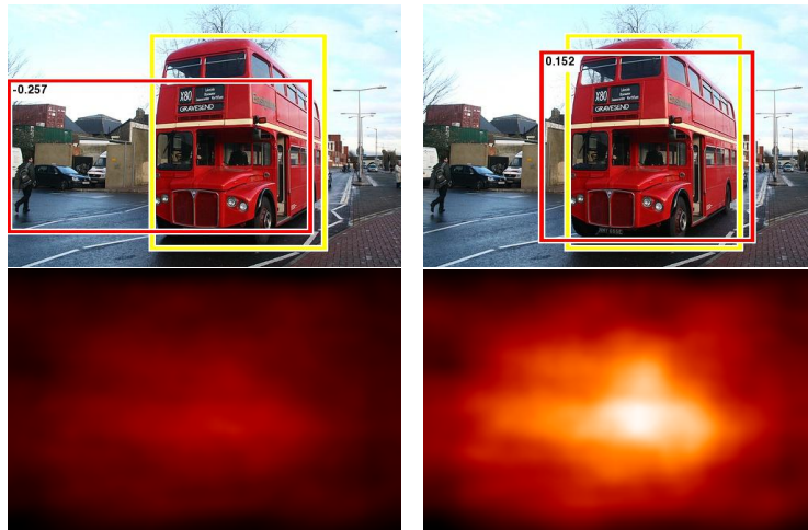
Figure 1: Screen shots of object detection results. This shows how our active learning approach improves object localization. The top left shows the highest scoring detection using only VOC 2007 data, whereas the top right shows the result after retraining with additional data obtained using our active learning interface. The bottom row shows associated confidence maps in the same scale. Note how the detection confidence increased and the peak position was shifted. Yellow boxes are the ground truth and red boxes are detections with the associated detection confidence.
