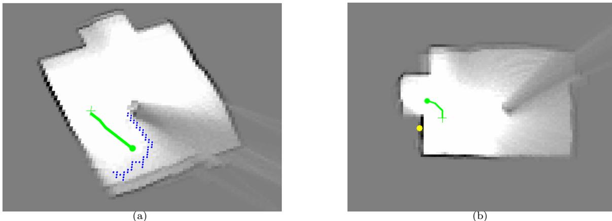
Fig. 4. Paths are planned to achieve numerous goals. (a) Path towards frontier of unexplored space (indicated by blue dots) allow for exploration. (b) A path to another clear view of an object (indicated by a yellow dot) can be used to obtain multiple views. Legend: + start of path. • end of path.
