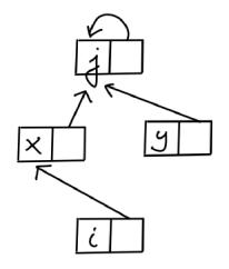
1. if we are dealing with a set of |S| = n elements, the find(x) operation requires up to O(n) to follow the pointers starting at x to reach the node (j in the above example) after which the set containing x is named.
