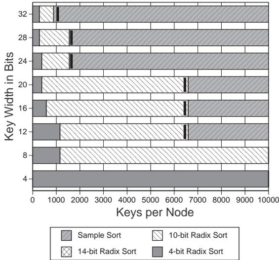
Figure 11: This plot shows the best algorithm for a given key width and keys per node for a 64-node CM-5. These regions are the predictions: the black bars denote the actual crossover point. The bars are omitted for clarity if the predicted crossover is within 0.5% of the actual crossover point. Thus, the models accurately predict the best algorithm. Note that 14-bit Radix Sort never wins.
