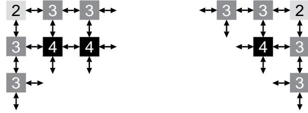
Figure 13: Boundary processors have fewer neighbors to communicate with than nodes in the center.
