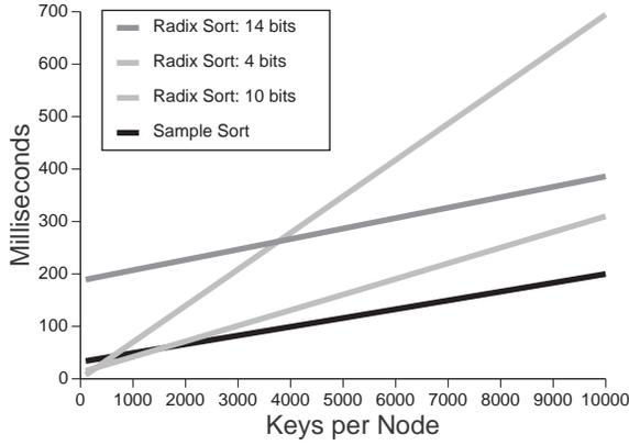
Figure 10: Sorting Performance on a 64-Node CM-5. This graph shows the performance of the four sorting algorithms for a 64-node CM-5 and 28-bit keys. Sample sort is the best for large problems, while the small-radix radix sorts work best for small problems.
