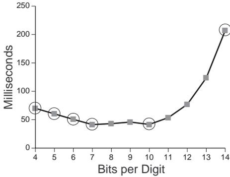
Figure 15: This graph plots the proposed composite model from equation (6) against the parameter (bits per digit). The graph has multiple minima and thus could lead to suboptimal values. Only the circled nodes are considered by the revised model of equation (7), which only has one minimum (at 7).
