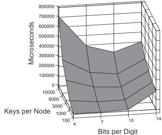
Figure 14: This graph plots the performance of radix sort on a 64-node CM-5 with 28-bit keys, versus the width of the digit in bits and the number of keys per node. For less than 1000 keys per node, the optimal width is 4 bits, around 1000 it is 7 bits, and above 1000 it is 10 bits. For large enough sorts, 14-bit digits would be optimal.
