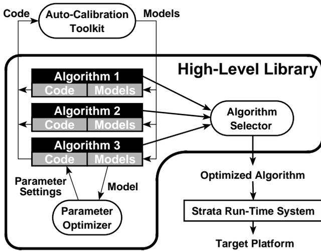
Figure 2: A high-level library consists of a set of algorithms each with code and models. The models used are automatically generated by the auto-calibration toolkit and are used for algorithm selection and parameter optimization. The selected algorithm is then compiled for the target platform using the optimized parameter settings.
