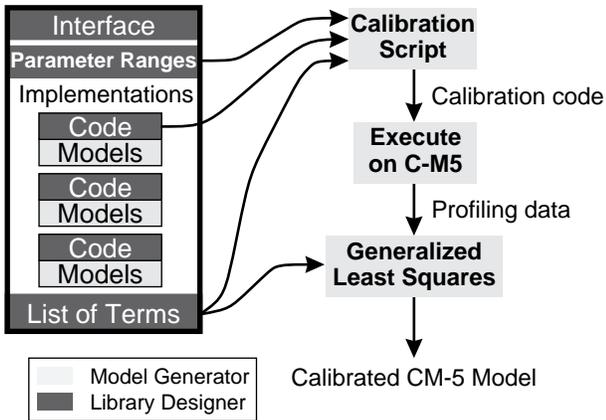
Figure 3: This block diagram describes the automatic generation of models via profiling and linear regression. The dark gray boxes indicate inputs provided by the library designer, while the light gray boxes are provided by the auto-calibration toolkit. Calibration code is generated from the code and the parameter ranges; upon execution this code produces the profiling data used to fit the models terms provided by the designer.
