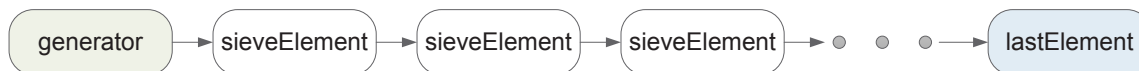
Figure 1: A pipeline of processes, where numbers generated by the generator are streamed through the chain to be processed by each element.
