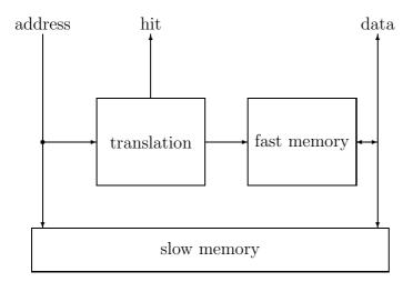
The translation is usually implemented by a contents-addressable memory that matches addresses accessed against the addresses (tags) which are cached. A *cache line* consists of one block of data, its address (tag), and the extra hardware needed to implement a CAM, in particular a tag comparator.
