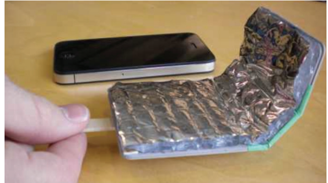
Figure 1: An early prototype ( Curl ) of a mobile device creating a biologically inspired life-like gesture.
