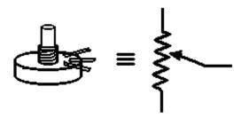
Pots are nice because they're cheap, and relatively low-noise (but see below). Pots are not so nice because there's scraping involved with use, and they can wear out. Also cheap ones can get dirty or wet and stop working pretty quickly.
