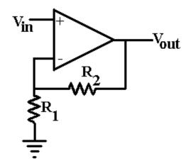
$$i_{R_1} = i_{R_2} = \frac{v_-}{R_1} = \frac{v_+}{R_1} = \frac{v_{in}}{R_1}$$
