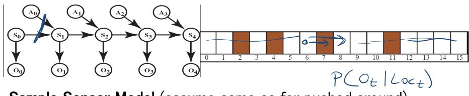
Sample Sensor Model (assume same as for pushed around) Sample Stochastic Dynamics:  $P(Loc_{t+1} | Action_t, Loc_t)$   $P(Loc_{t+1} = L) Action_t = goRight, Loc_t = L) = 0.1$   $P(Loc_{t+1} = L+1 | Action_t = goRight, Loc_t = L) = 0.8$   $P(Loc_{t+1} = L + 2 | Action_t = goRight, Loc_t = L) = 0.074$  $P(Loc_{t+1} = L' | Action_t = goRight, Loc_t = L) = 0.002$  for all other locations L'
