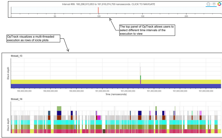
Fig. 16. OpTrack is part of WiredTiger. It visualizes per-thread call stacks, breaking up the timeline across 240 individual pages. A developer selects the page to view from the top panel.
