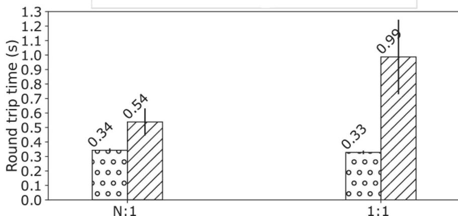
**Fig. 12** Sock-shop non-instrumented (Kubernetes) versus instrumented (Kubernetes)
