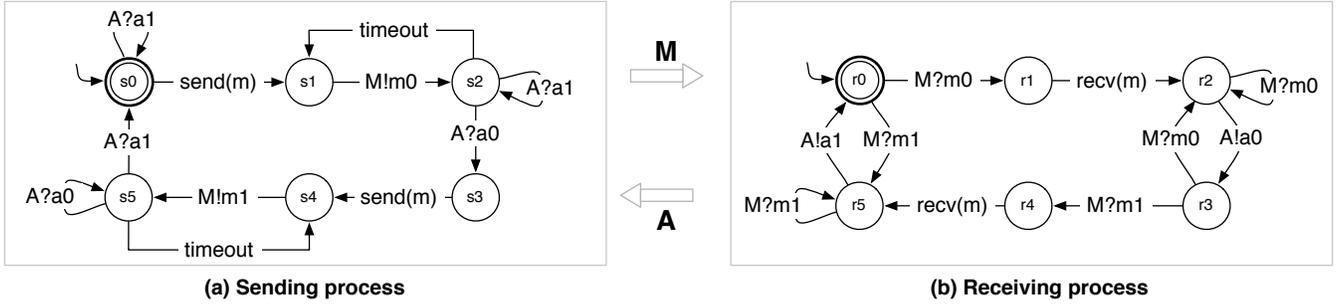
Figure 1: A CFSM model of the alternating bit protocol with (a) sending process model, and (b) receiving process model. The sender transmits messages to the receiver using queue  $M$ , and the receiver sends acknowledgments to the sender using queue  $A$ . Event  $Q!x$  means enqueue message  $x$  into queue  $Q$ , and event  $Q?x$  means dequeue message  $x$  from the head of the queue  $Q$ .
