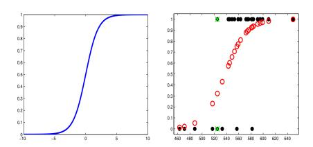
(Left) logistic or sigmoid function (Right) logistic regression for x=SAT score and y=pass/fail class (solid black dots are the data), open red circles are predicted probabilities.
