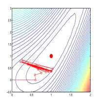
Gradient descent on a simple function, starting from (0,0) for 20 steps using  $\eta=0.1$  (left) and  $\eta=0.6$  (right)
