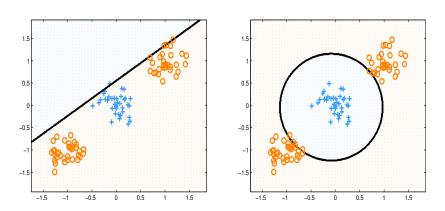
(left) Logistic regression in the original feature space  $\mathbf{x}=(x_1,x_2)$ . (right) Logistic regression obtained after performing a 2nd degree poly expansion  $\Phi\left(\mathbf{x}\right)=\left(1,x_1,x_2,x_1^2,x_2^2\right)$ .
