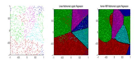
(left) Some 5 class data in 2d (center) Multinomial logistic regression in the original feature space  $\mathbf{x}=(x_1,x_2)$  (right) RBF basis functions with bandwidth 1 using m=1+N. We use all the data points as centers.
